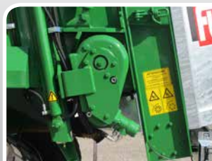
Riduttori maggiorati con attacco a millerighe Increased gearboxes with splined connection
