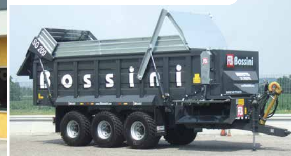
Cassone altezza standard +soprasponde 50 cm Standard container with extension sides 50 cm
