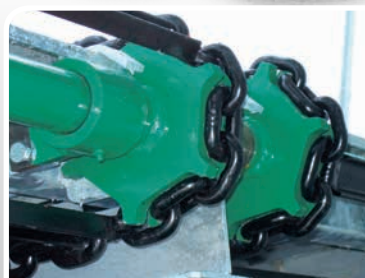
Catene speciali al nichel-cromo anti-usura e anti-stiramento Special nickel-chrome chains without wear and without stretching
