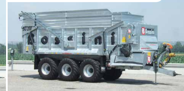
Cassone altezza standard +soprasponde 50+35 cm Standard container with extension sides 50+35 cm
