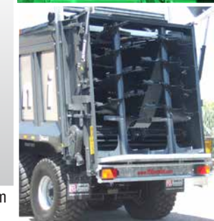
Rulli a coclea da 2100 mm Beaters with spiral h 2100 mm
