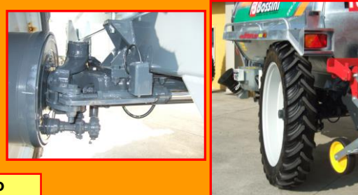
Assale sterzante comandato dalla trattore con cilindro idraulico (per gancio di traino alto e carreggiata larga) Steering axle commanded by the tractor with hydraulic cylinder (for high eyelet and wide distance between the tires)
