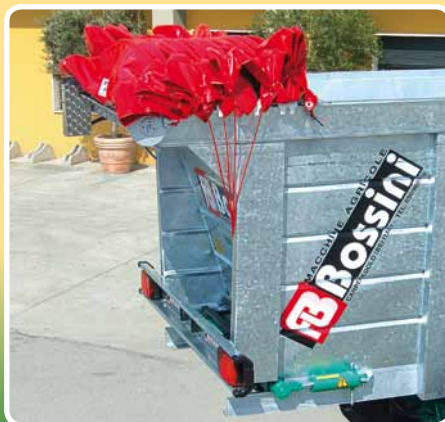
Copertura in PVC ad apertura anteriore o posteriore a comando manuale o in cabina PVC cover to open in the front or rear with manual or in the cabin control
