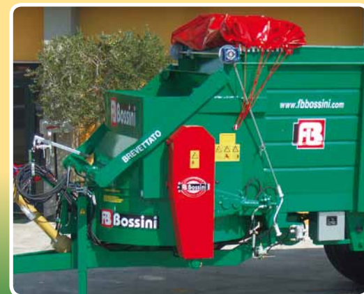
Copertura in PVC ad apertura anteriore o posteriore a comando manuale o in cabina PVC cover to open in the front or rear with manual or in the cabin control
