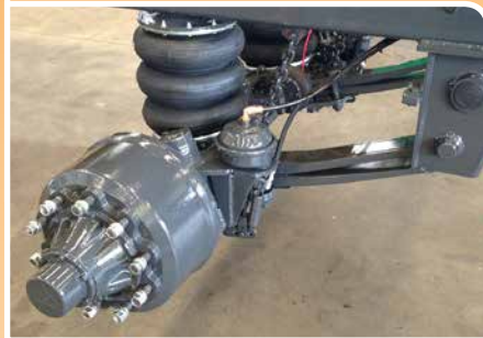
Frenatura a tamburo con camma ad evolvente e masse frenanti omologate fino a 105 Km/h Brake drum with cam involute and braking approved until 105 Km / h
