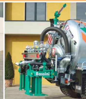
Interratore a 6 ancore snodate, fissato al telaio Injector to 6 foldaway exits, fixed to the chassis
