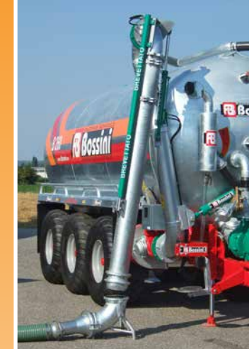
Braccio con sfera in testa Arm with ball joint to the end
