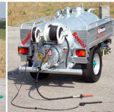
Naspo alimentato dalla pompa centrifuga e barra lava strade Hose reel powered to the centrifugal pump and bar washes streets
