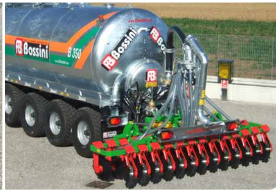
Barra rasoterra applicata al sollevatore per varie dischiere Bar applied to the linkage for various disc equipment
