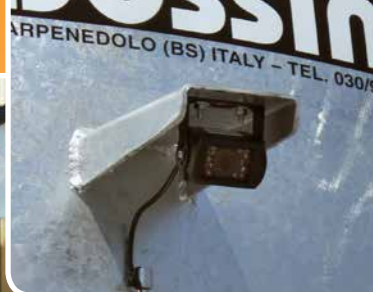
Telecamera ad infrarossi con monitor LCD sulla trattrice Infrared camera with LCD monitor on the tractor
