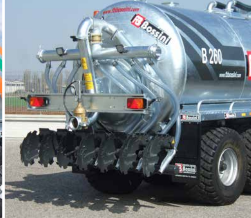
Dischiera 2,55 m fissata al telaio Disc equipment 2,55 m fixed to the chassis
