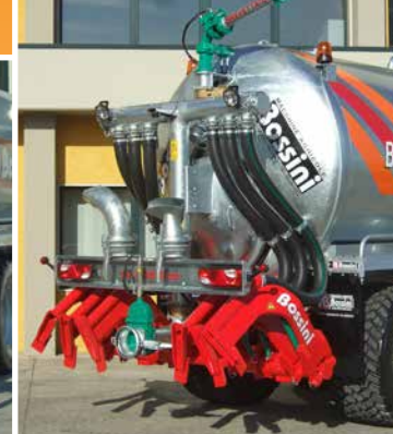
Interratore a 6 ancore snodate, fissato al telaio Injector to 6 foldaway exits, fixed to the chassis
