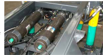
Accumulatori ad azoto a membrana o doppia camera Nitrogen accumulators with membrane or piston-type
