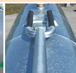
Doppia valvola primaria in centro al serbatoio Double primary valves in the center of the tank
