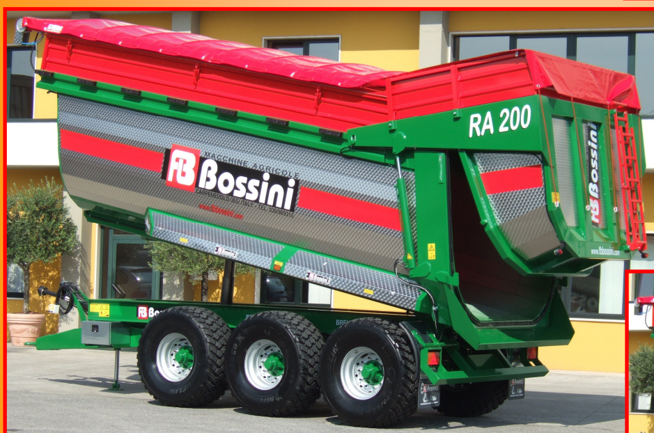
RA200/6 con cassone Inox + Sopra-sponde cm 50 e copertura in PVC RA200/6 with Inox container + over side cm 50 and plastic ground cloth
