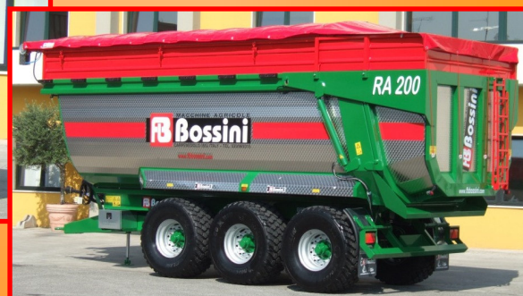
RA200/6 con cassone Inox + Sopra-sponde cm 50 e copertura in PVC RA200/6 with Inox container + over side cm 50 and plastic ground cloth
